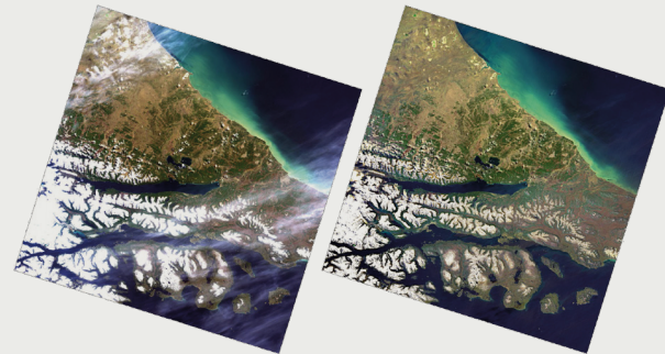
ATCOR-3 correction and haze removal for Sentinel-2.
