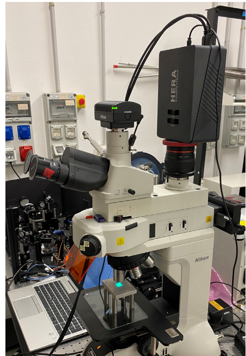
Figure 3: HERA VIS-NIR coupled to a Nikon LV100 upright microscope.
