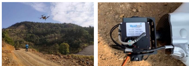
Figure 1. Unmanned aerial vehicle (UAV) flight status (left) and onboard Headwall Nano-Hyperspec imaging spectrometer (right)
