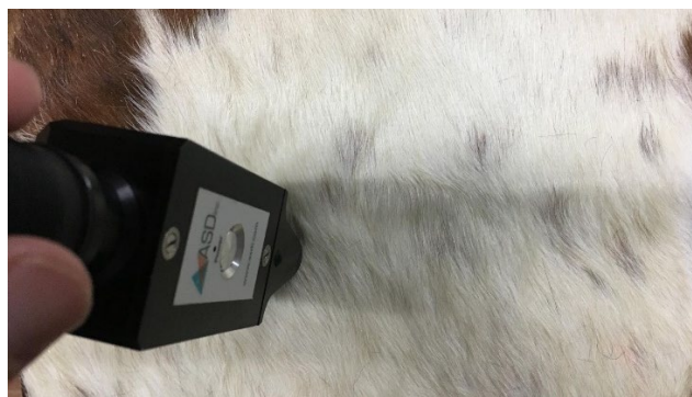
Figure 1. Measurement of animal hide with ASD spectroradiometer with Contact Probe fore-optic.
