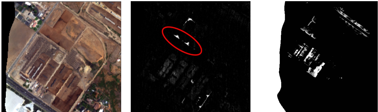
Figure 4. Sub-study area providing example detection results. (Left): true-color image. (Center): stretched ACE plane for dark-toned hide signature; circled area references Fig 6. (Right): stretched SAM rule image of waste material signature.
