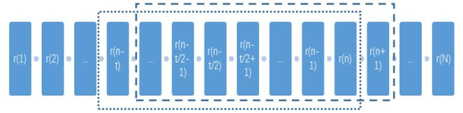
Fig. 1 Sliding array RX detection algorithm
