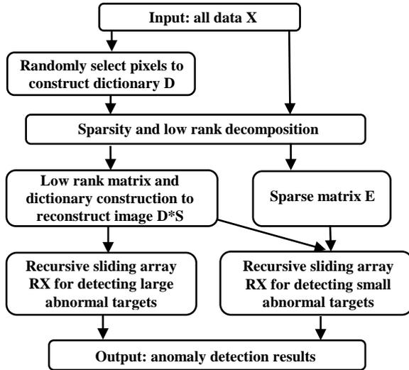
Fig. 4 The process of multi-scale anomaly detection in hyperspectral image based on sparse and low rank decomposition
