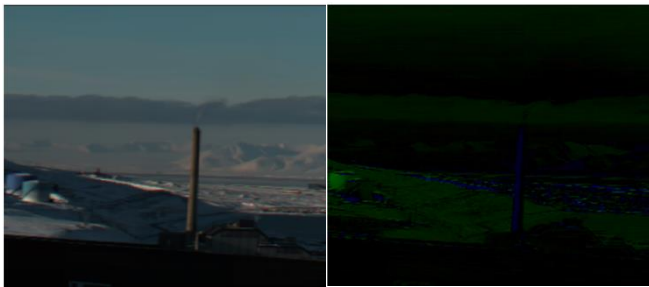
Fig. 4: Compressed H.265 QP30 RGB-image (MNC 121) (L) and the compressed image subtracted from the reference image (MNC 83) (R).
