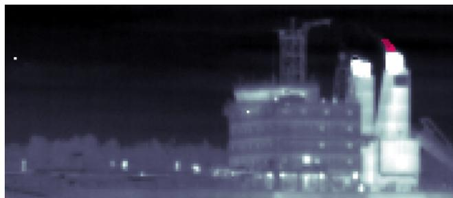
**Figure 2** SO<sub>2</sub> detection of a moving ship. The ship is moving eastward (toward the left) on the Saint-Lawrence seaway.
