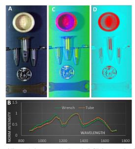
**Figure 4 Example image set. A: Pseudo RGB image using** image of training data made in SWIR 1094 nm (red), 1301 (green), 1475 nm (blue). B: Normalized spectra of the wrench and the tube from the selected region of interests. Spectral correlation is 0.93; C: PCA in pseudo RGB: component 1 (red), component 2 (green), component 3 (blue). D: Endmembers in pseudo RGB (see text).
