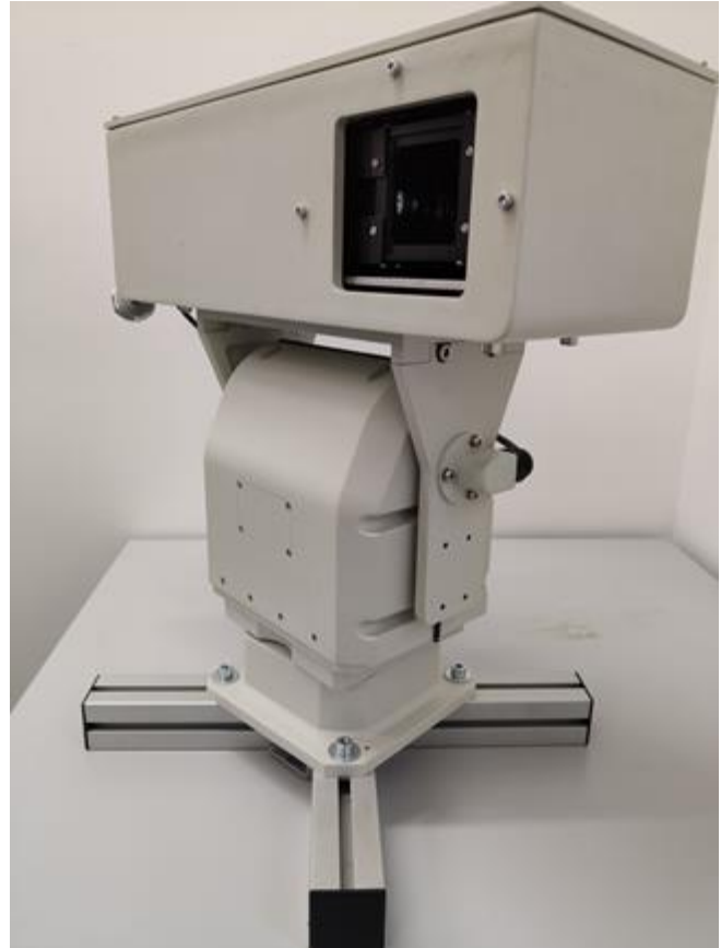
Fig. 2. The RODES system in the durable body with a pan-tilt system.
